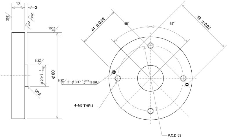
According to the diagram above, open mounting holes for the robot from the force sensor mounting side.
